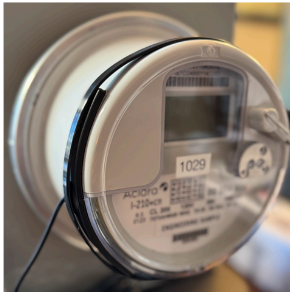
Figure 2. External Fix-Up Antenna installed on Smart Meter.
