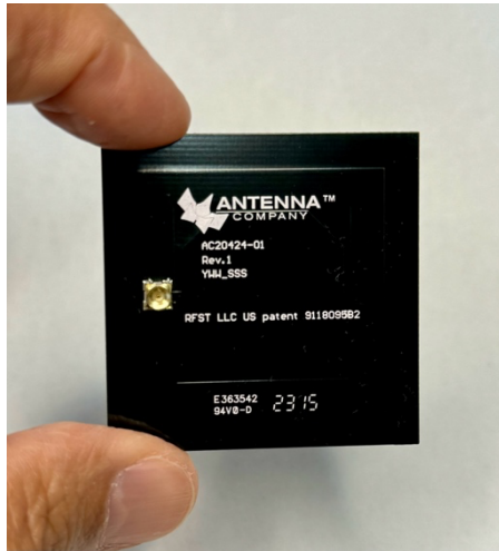
Figure 1.0 AC20424-01 RF Coupler/Isolation Circuit*
